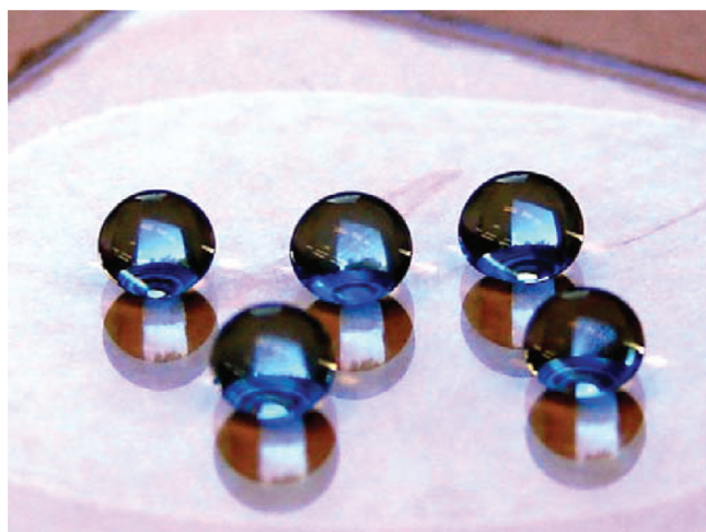
Figure 7. Optical photographs of water droplets (>10 \mu L) on F-SiO 2 NP-coated polyester fabric. A small amount of dimethyl methylene blue dye was dissolved in water for illustration purpose.
